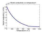
Fig. 2.2. Temperature dependence of the electric conductivity  $\sigma$
