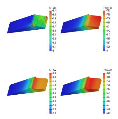
Fig. 6.3. History of the inductive heating process: Temperature distribution in a quarter-tooth at t=0.04~s (top left), t=0.80~s (top right), t=1.40~s (bottom left), and t=2.00~s (bottom right).
