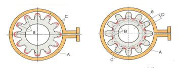
Fig. 1.1. Induction heating at high frequency (left) and medium frequency (right). At high frequency only the tips of the teeth are heated up, whereas at medium frequency most heating occurs at the interstitial space between the teeth (cf. region C in the left and right figure)
