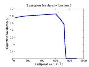
Fig. 2.1. Temperature dependence of the function  $\alpha$  and the saturation flux density  $\beta$  in the generalized Fröhlich's model.
