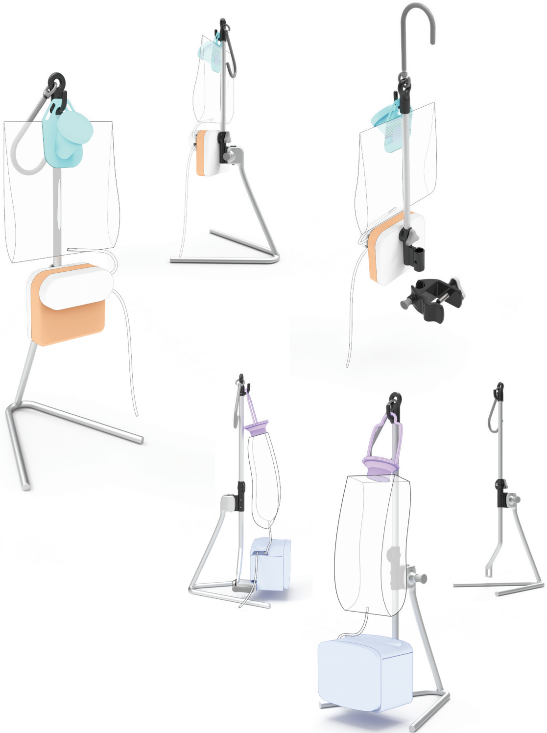
Figure 54. Final design in use with Infinity pump and Kangaroo Joey pump
