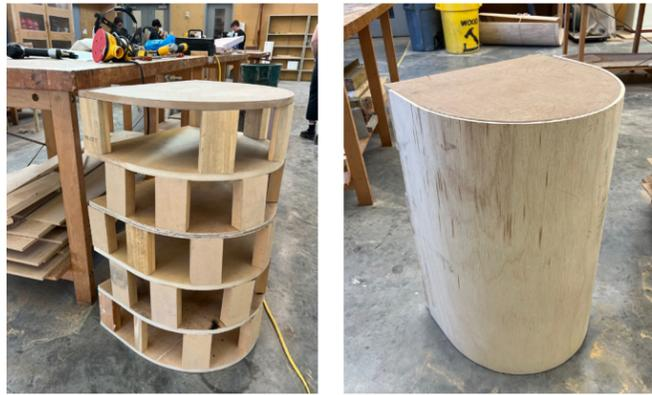
Step 1: Build the mold out of MDF and bendable plywood, then apply saran wrap.
