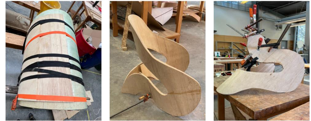
Step 4: Using the same mold, laminate the legs and trim legs to shape. Then, glue to the main body of the chair.
